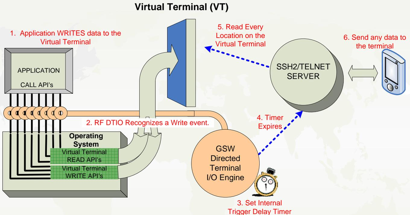
Since the RF DTIO “hooks” all Console I/O API’s it already has the knowledge every time the application reads or writes data to the Virtual Terminal. Two main cases to review are when the application Read and when the application Writes.
