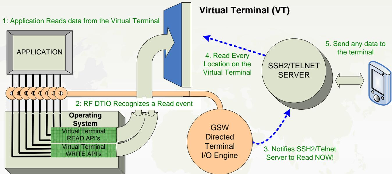
Let's look at what happens when the application performs a read. Usually (but not always) when an application's writes are complete, a read is performed to see if there is a response from the operator. If the application performs a read after completing screen updates then RF DTIO can be **optionally configured** to provide further performance gains.
