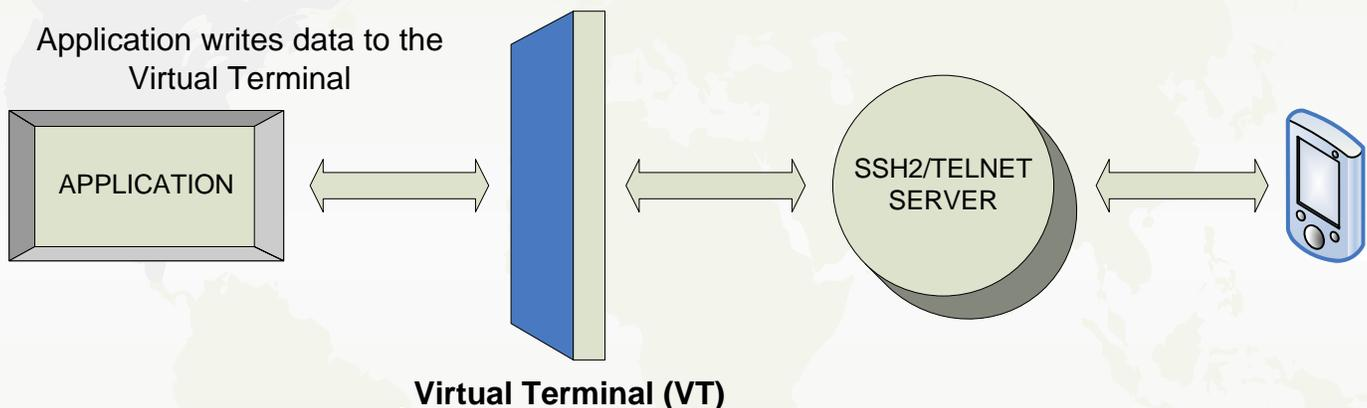
*Note: The Virtual Terminal is the Console Window maintained by the SSH2/Telnet command prompt and accessed through Windows Win32 Console API's*
